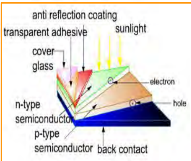
Layers of a typical PV module
